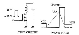
$$\begin{aligned} R_G &= 25~\Omega \\ V_{DD} &= 90~V,~L = 4.59~mH \end{aligned} \qquad E_{AS} &= \frac{1}{2} \cdot L \cdot I^2 \cdot \left( \frac{B_{VDSS}}{B_{VDSS} - V_{DD}} \right) \end{aligned}$$
